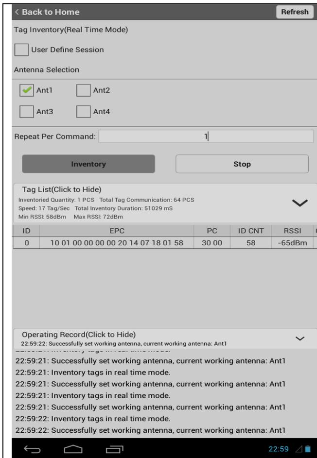
3. Close the tag, the Tag list will show the data change, the means that the device are read the UHF RFID tag successfully.
